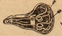
Rust is liable to get into the springs of the saddle without being observed.
