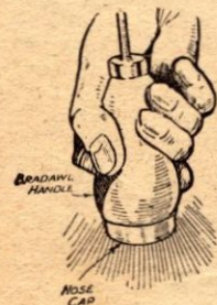
Fig. A.—If the nose cap will not fit over the nose of the fuselage, open it a little with the round end of a bradawl handle or similar tool.
