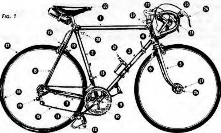
1. Top tube, 2. Seat tube, 3. Down tube, 4. Head tube, 5. Front fork, 6. Front fork crown, 7. Chainstay, 8. Seatstay, 9. Bottom bracket, 10. Chainwheel, 11. Pedal, 12. Toeclip, 13. Chainwheel derailer, 14. Rear derailer, 15. Chain, 16. Rim, 17. Tyre, 18. Brake, 19. Flint catcher, 20. Saddle, 21. Feeding bottle carrier, 22. Handlebar stem, 23. Handlebar, 24. Brake lever, 25. Rubber shock absorber ('climbing rubber'), 26. Hub, 27. Wingnut, 28. Seat tube angle, 29. Head tube angle.
