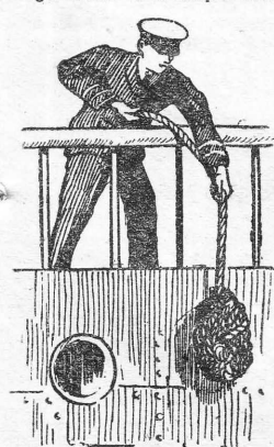
To prevent a ship from damaging its sides against the wharf, a rope fender is used.
