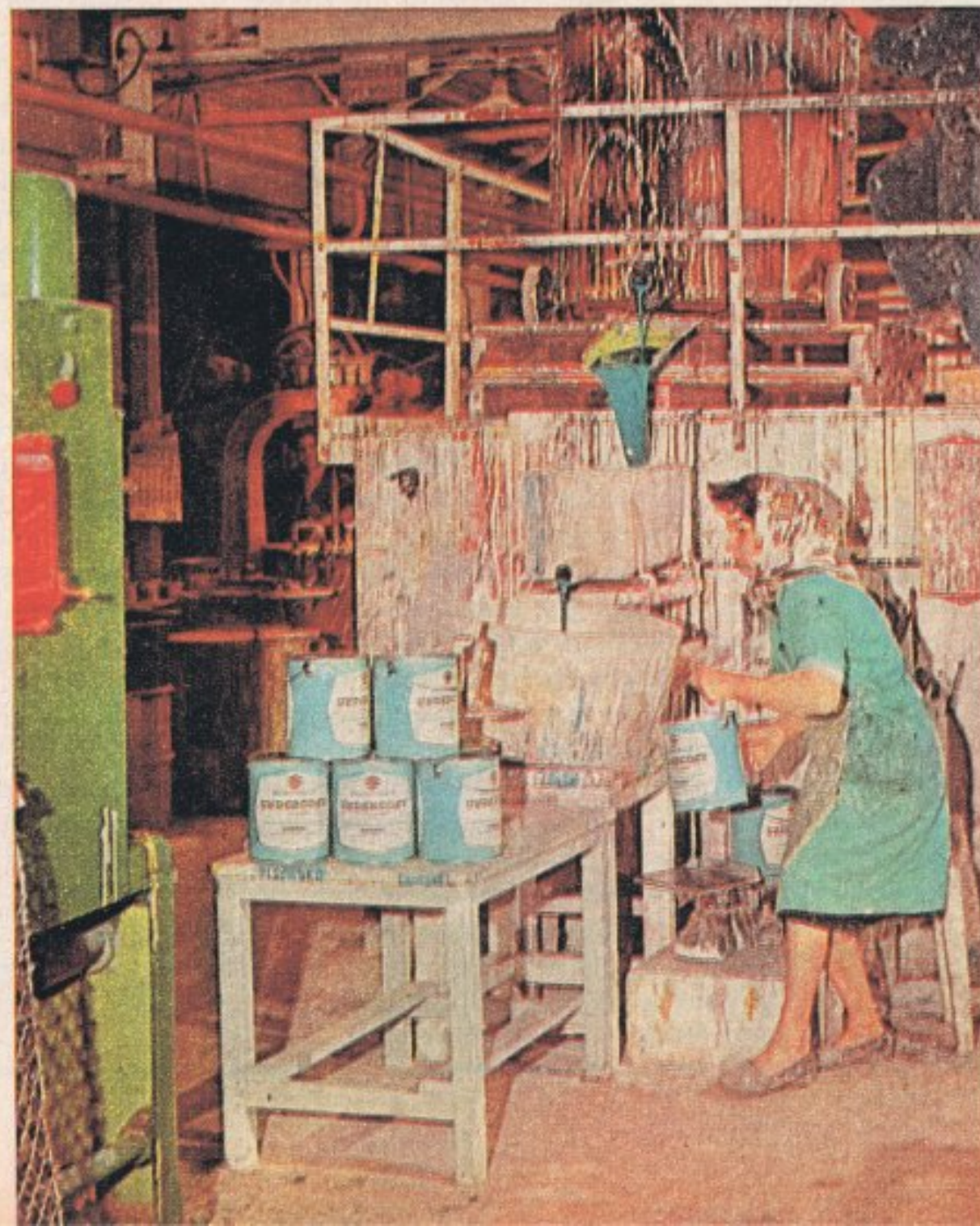
To measure stickiness a blob of paint is placed on a metal surface (above the girl's left hand) and then ground by a revolving screw. The resistance the screw meets to its spin measures stickiness.
