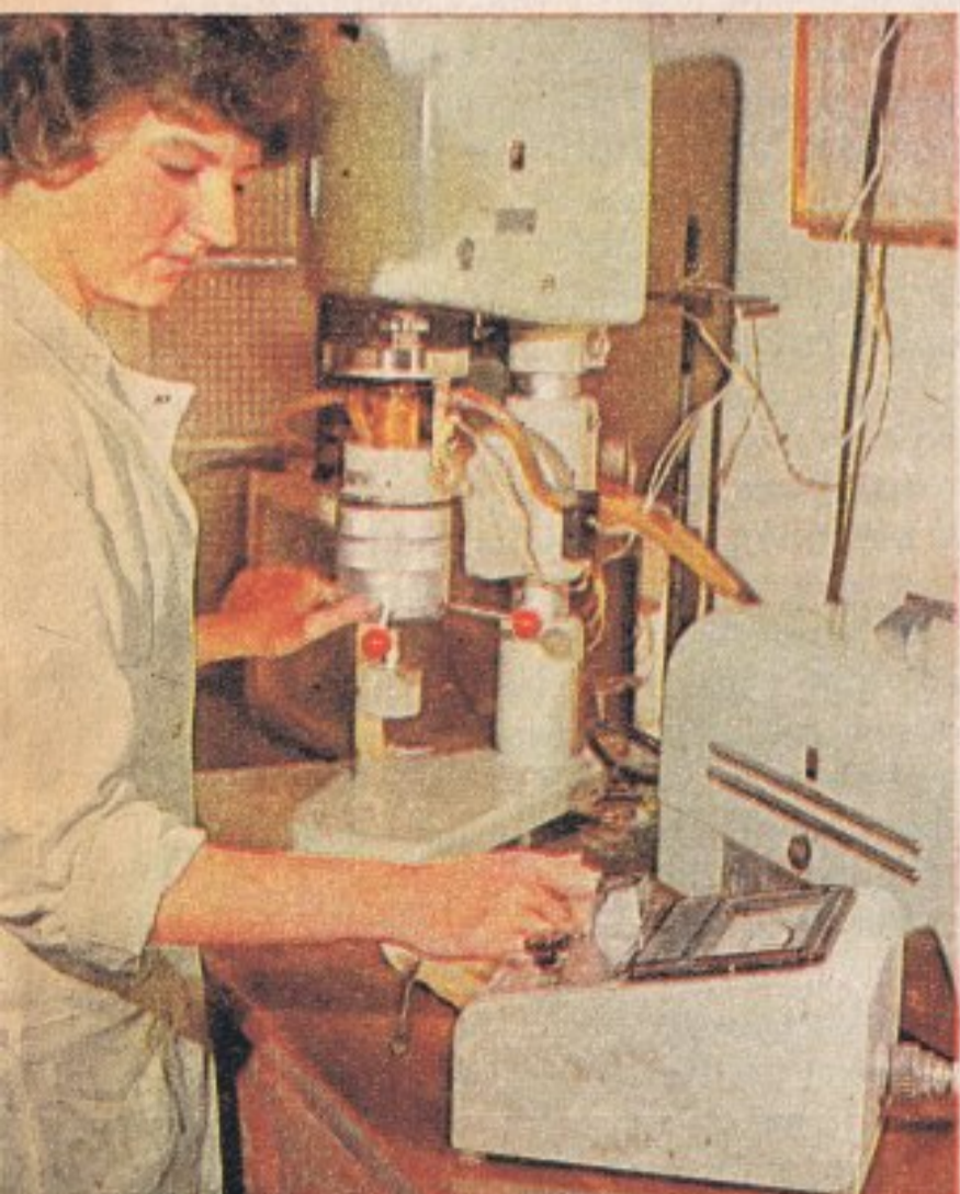
To measure stickiness a blob of paint is placed on a metal surface (above the girl's left hand) and then ground by a revolving screw. The resistance the screw meets to its spin measures stickiness.
