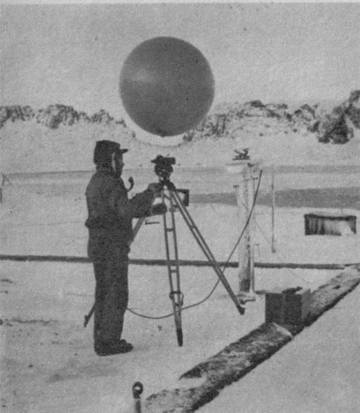
METEOROLOGY At Deception Island in the South Shetlands a balloon is launched to track the course of the winds. Its route will be tracked by a theodolite.
