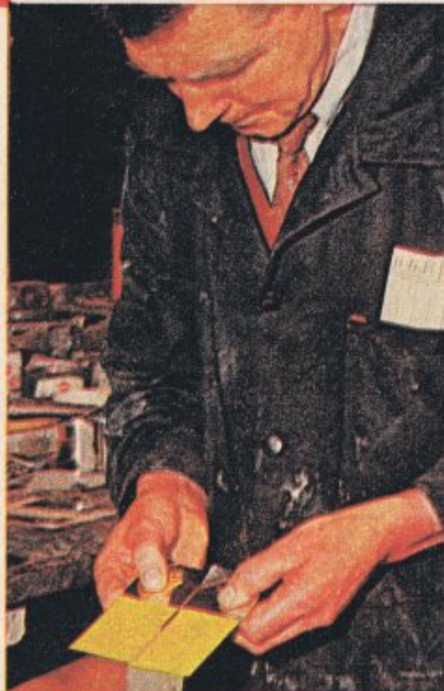
The solvent is added to the paste from the pugging mills, and the paint is then tested for its colour. A sample is painted on a piece of glass and compared with a sample of the correct colour which is on another piece of glass (left). The matching is done by eye and requires great skill (above). Pigments are then added to lighten or darken the paint.
