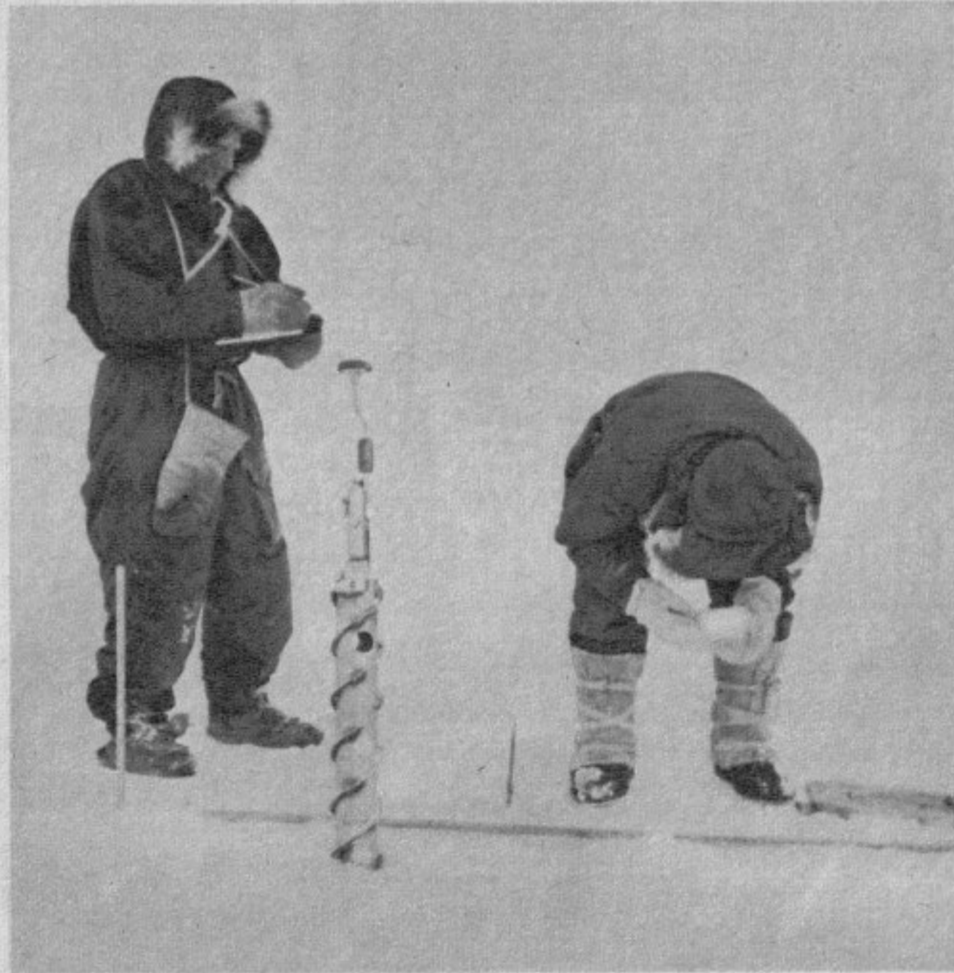
GLACIOLOGY Many scientists in the Antarctic are studying the ice itself, not only on the surface but far below. This special instrument bores into the ice and brings specimens to the surface.
