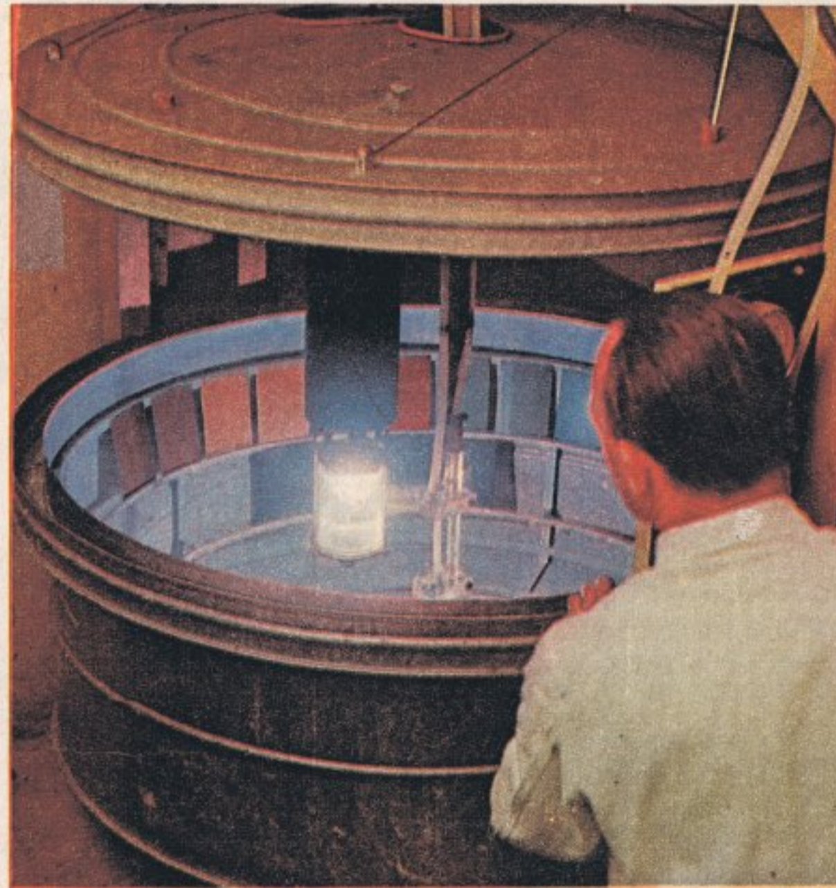
All the paints have to be tested very carefully to see how well they stand up to the weather. A sample of the paint is brushed on to a panel, and placed in a "weatherometer." The panel is then subjected to intense ultraviolet light (which is equivalent to sunlight) and rain. Tiles are also exposed to the natural atmosphere on the roof of the factory.
