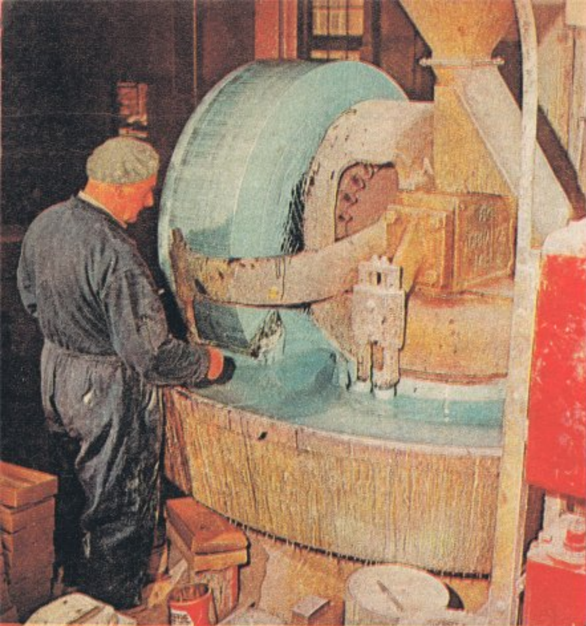
The pigments, which are obtained from a supplier, and the synthetic resins, which are made in the factory, are ground together by a "pugging mill." The right quantities of pigments needed to make a particular colour are worked out in the factory's laboratories.
