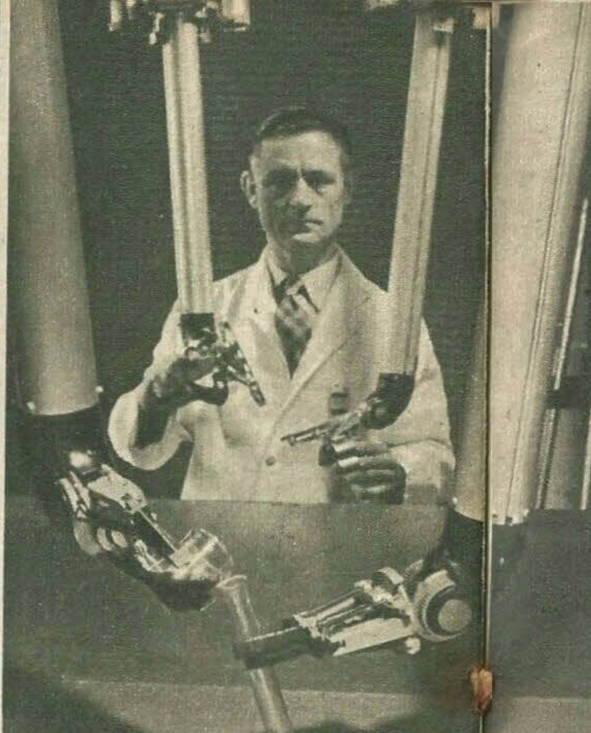
To protect himself against the deadly radiation, this technician is using robot fingers to handle radio-active material.
