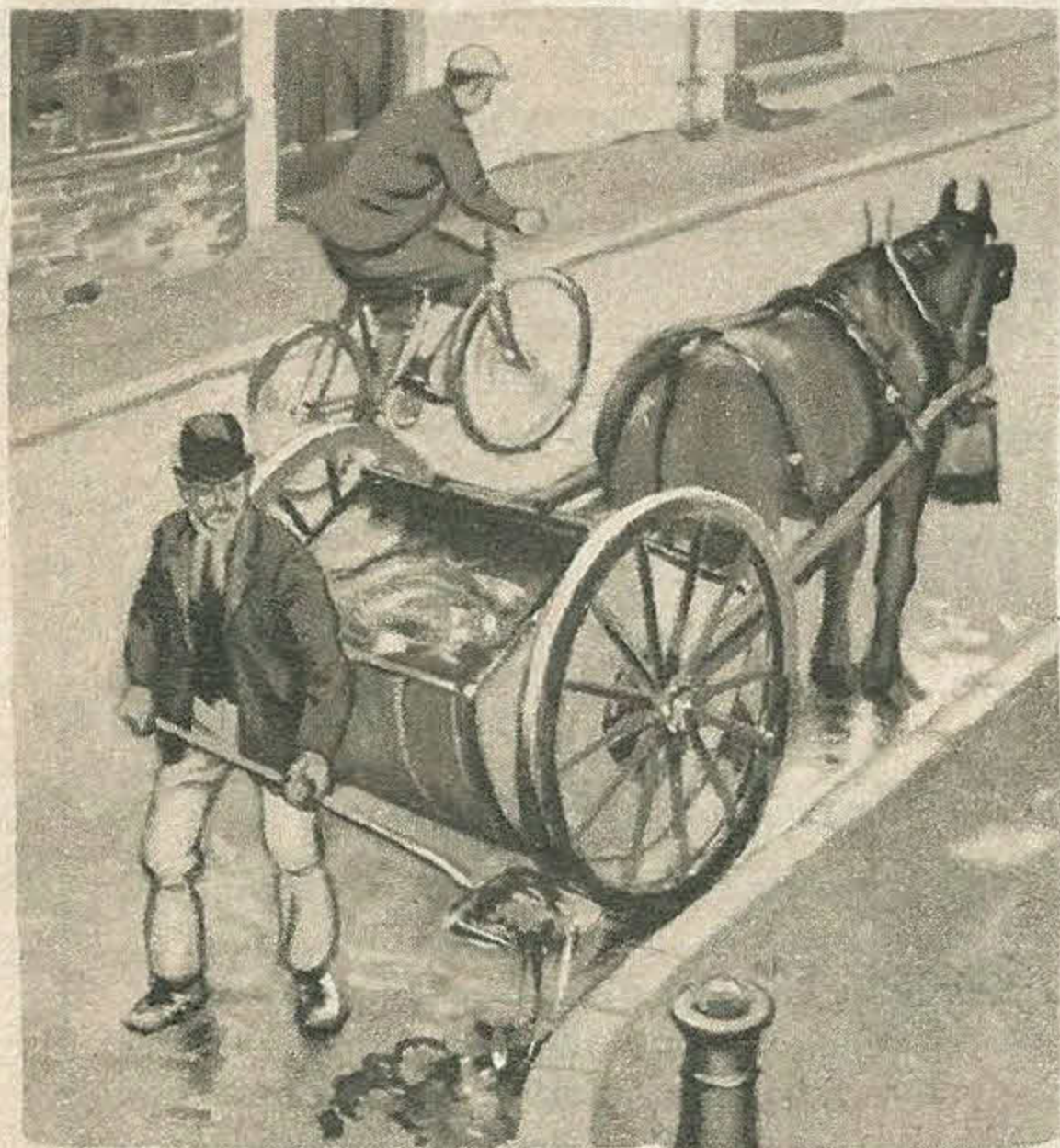
The mud-cart, or "muck-cart" as it was called, was a familiar sight about 1910, carrying away mud and sweepings from the gutter. This cart was the first attempt at mechanized road cleansing.
