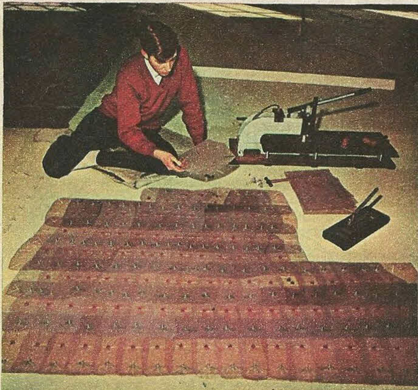
The templates are carefully pinned together so that they make a perfect mosaic of the area. The correct position of each pinprick is measured off, and all the positions are transferred on to the map which is being made of the area. The overlap of the photos allows landmarks to be double-checked.
