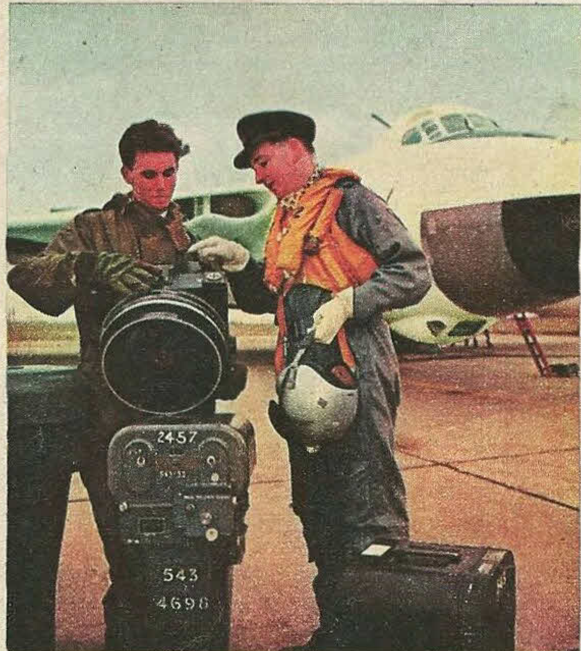
The survey cameras take one photo every twenty-five seconds. As the plane flies at about 500 m.p.h., there is a 60 per cent overlap between two successive photos. Thus each area is covered twice.
