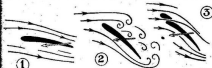
Fig. 1.—The air is flowing smoothly round the aeroplane's wing (shown in section), and lifting it. Fig. 2.—The air here is not so steady, and the air starts eddying behind it and the "stall" decreases rapidly. Fig. 3.—How the Hardy Page started wing warps. Here the air has opened, restoring the smooth air-flow.
