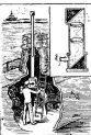
The modern periscope—the eye of the submarine—is like a long telescope with a clever arrangement of lenses and mirrors, as shown in the smaller illustration. In this latter drawing an observer is turning the periscope's head in the desired direction by means of a lever.
