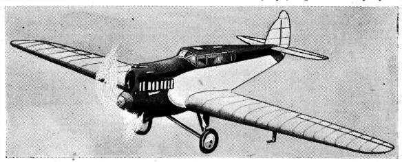
Particularly designed for the private owner, it is quite fast, cruising at 112 m.p.h., with 130 m.p.h. as maximum speed. The cabin is roomy, with large windows in the sides and roof, and the view from the pilot's seat is very good. The petrol is carried in the wings. The engine is a Cirrus-Hermes, neatly cowled in.
