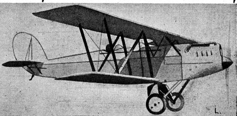
pronounced sweep-back. The seats being well clear of the wings allow of a very good all-round view. So here we have several unorthodox features, almost any of which would enable us at once to pick the machine
