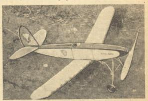
It is powered with ten strands of 4-inch flat rubber, and its weight is 54
