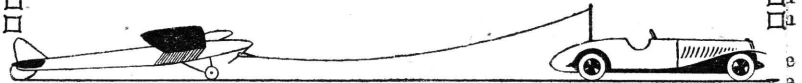
Fig. 2.—How a model glider can be towed behind a clockwork model car, the tow-line being fixed to a small upright in the back of the car.
