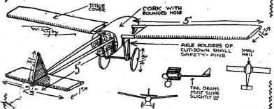
With small pieces of split cane make the frameworks for the rudder and the main-planes, and glue and bind them to the ends of the tail beams. Cover the main-planes, rudder, and tail-planes with grease-paper or tissue-paper
