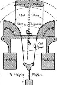
attached. The steel straps hanging from the top of the machine are shortened, since they are pulled around the segments, and consequently, since the distance between the frame of the machine and the horizontal bar has been lessened, the latter rises.
