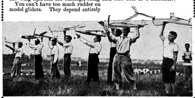
on air-currents flowing past them, and they must be constantly headed into the wind. Notice how most of the models in the photo have very slim fuselages—to save weight and air resistance. For the same reason, some of the models are not fitted with undercarriages or landing gear.
