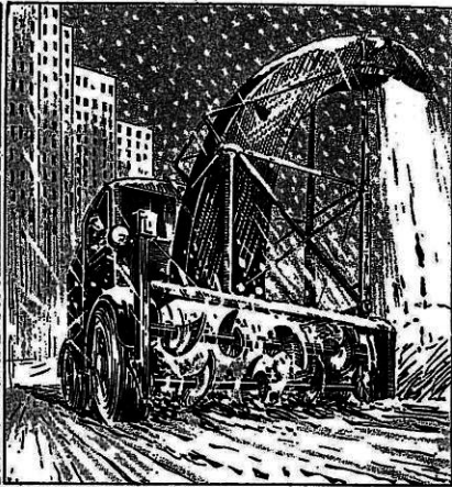
Here's the way to get a snow-covered road cleared quickly. Machine is like a giant vacuum cleaner. Special rollers gather up the snow and it is passed into a big chute where it is blown up through a curved shaft and deposited by the roadside. Much the same idea has been tried on the railway.
