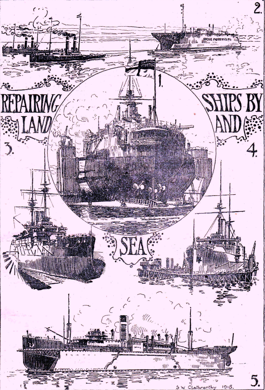
1. British Super-Dreadnought lifted high and dry in floating-dock for cleaning and repairs. 2. British-built floating-dock for South American port in tow of Dutch ocean-going tugs. 3. British pre-Dreadnought Battleship in graving-dock at naval port. 4. Battleship entering floating-dock submerged for her reception. 5. Ocean tramp undergoing repair in floating-dock.
